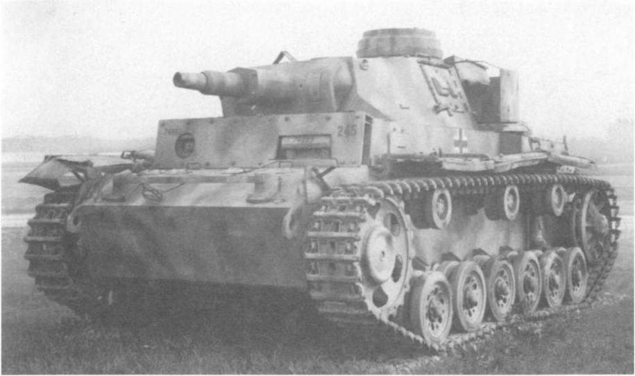
Early "Organization D" Tiger battalions were partially equipped with Panzer IIIs, Version ( Ausführung ) N. This model of the Panzer III was armed with a low-velocity 75 mm L/24 gun. ( Patton Museum of Cavalry and Armor )
