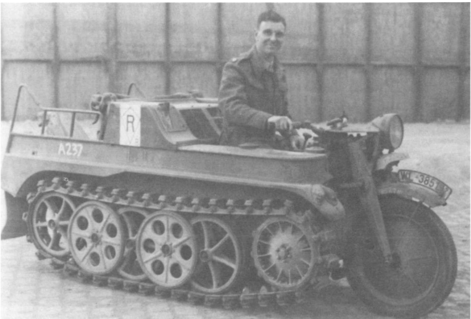
A Sonderkraftfahrzeug (SdKfz) 2 Kettenrad . Six Kettenräder were authorized in the scout and engineer platoon of Organization E battalions. Intended for reconnaissance missions, each one carried two men. ( Patton Museum of Cavalry and Armor )
