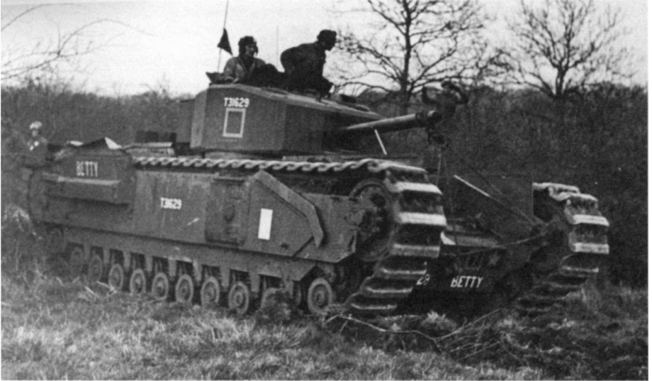
A Churchill III of the 14th Canadian Tank Regiment. Heavily armored but slow, this Churchill is armed with a 6-pounder (57mm) main gun. Later variants were even more heavily armored and were reequipped with a 75mm main gun.
