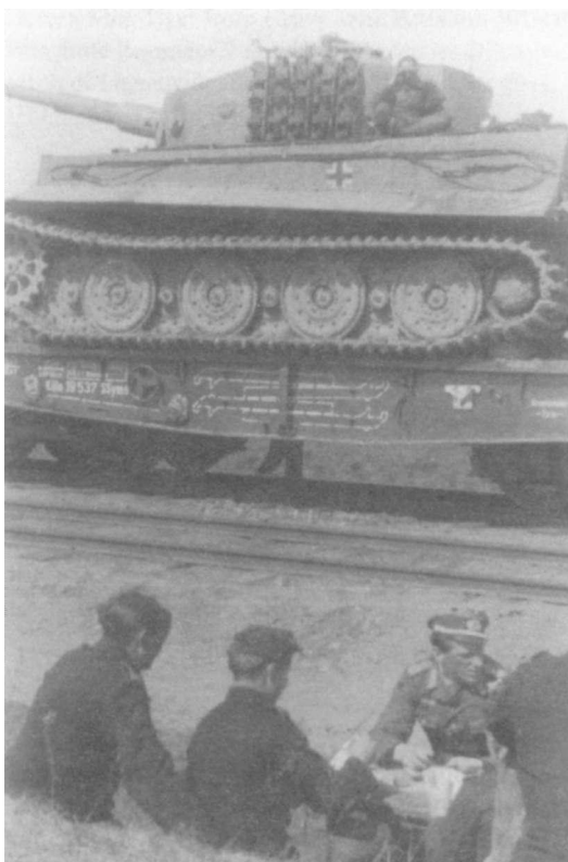
Tigers were prone to an unusually high breakdown rate when traveling even relatively short distances on roads, so rail movement was essential for long-distance transfers. Of course, rail movement included its own special challenges, including the need to use special narrow tracks on every tank, and a paucity of the unique rail cars which could carry Tigers. Here, a Tiger is entrained on the reinforced Ssyms rail car, awaiting transport to the front, March 1944. This particular tank is from the 3d Company, Heavy Tank Battalion 505. March 1944—Leutnant Hilbig is facing the camera. (Dale Ritter Collection)
