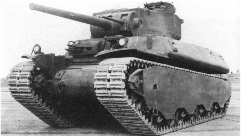
The T1E2 (later, M6 series) Heavy Tank was an early US Army design for a heavy tank. The first prototypes were tested on the day after the attack on Pearl Harbor. In contrast, the first Tigers were not available for testing until over five September 1942. Armed with a three-inch (76mm) gun and well armored, the design never saw combat.
