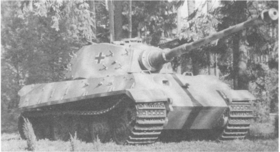
The King Tiger tank, also called the "Tiger II" or the "Royal Tiger." Appearing in 1944, it was the successor to the Tiger in every way: its main gun was even more lethal; its armor thicker and better designed; its motor and drive train more fragile; and its fuel consumption greater. (Patton Museum of Cavalry and Armor)
